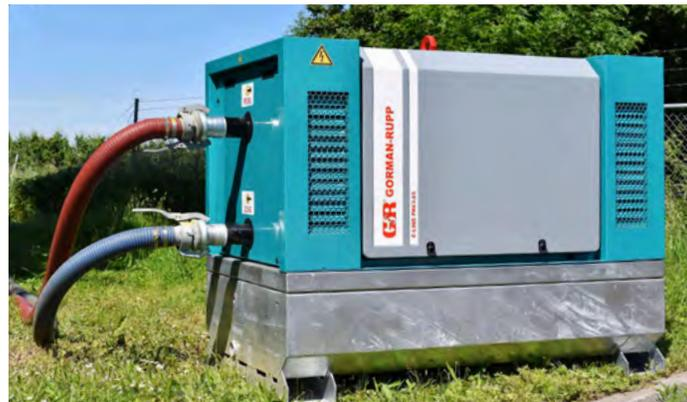
**ELECTRIFICATION OF MOBILE PUMP SETS.** We are developing more electric driven portable units for sale and rental. One of our latest developments is the E-Line, the first fully integrated electric drive solution in which a pump set can be connected to a regular construction power point, a mobile battery pack, or even to a car charger.
